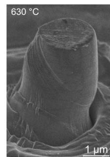
This tip heating capability also permitted thermal stability to be quickly re-established in site-specific microcompression experiments. This allowed compression of nickel superalloy micropillars up to sample temperatures of 630°C with very low levels of oxidation after 48 h. Furthermore, the measured Young moduli, yield and flow stresses were consistent with literature data.
