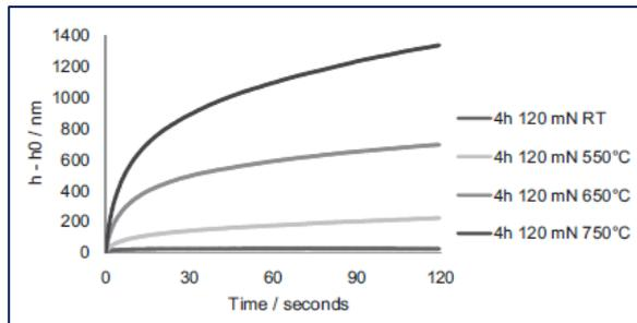
**Fig 3: High temperature creep data for G18 aged for 4 hours**
