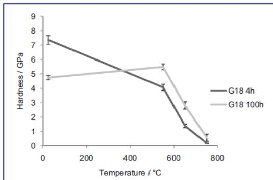
Results showed a decrease in reduced modulus with increasing temperature, with significant decrease above the glass transition temperature, while hardness generally decreased with increasing temperature (Fig 2).
